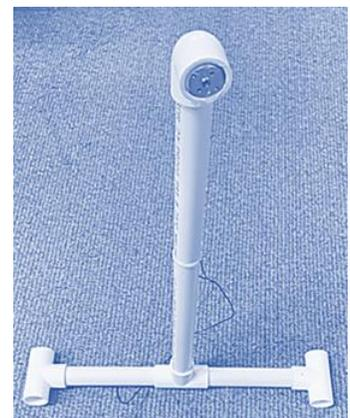
3. Attach "T" connectors to the end of both 6" pipes.
